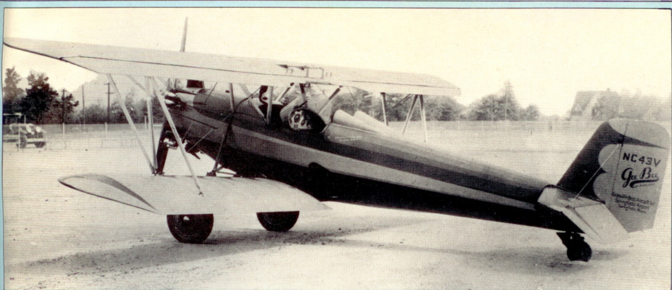
The prototype A on skis with its final engine, a 100-hp Kinner K-5 (above left). The production Gee Bee A (below) had a wider fuselage than the prototype and deleted the lower wing flaps, but was otherwise identical. Note the wider spacing of the headrests and the enlarged double-contour windshield. Later modifications in the engine mounts moved the engine forward six inches to improve lateral stability. One unique feature was the interchangeability of all the wing panels and stabilizers. The later A's also had full-span "flaperons" on the top wing (above), brakes on each set of rudder pedals, and a swivelling tailwheel that locked for takeoff.
